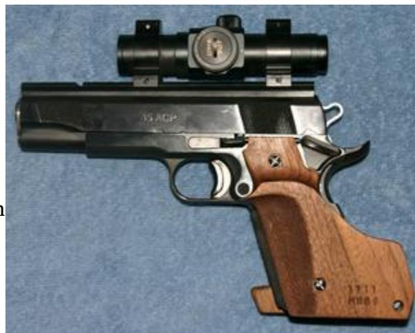
While mounting the dot sight directly upon the slide is the preferred method, it may also be mounted to a frame (bridge) mount, such as the Clark Scope Doctor mount.
