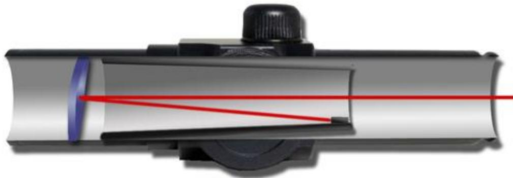
A cutaway of a typical red dot sight showing the concave reflective lens and LED.
