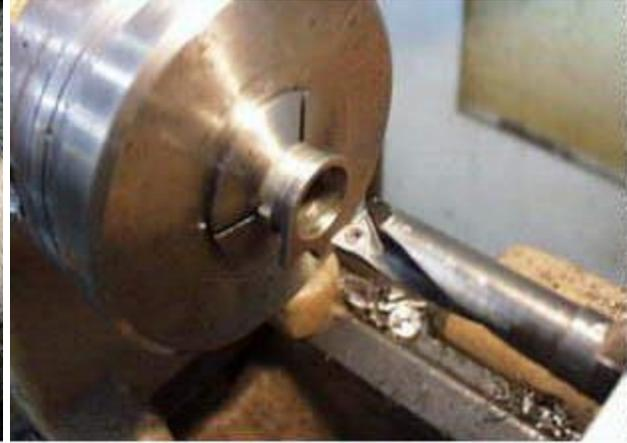
**Figure 11: The National Match bushing being machined to .001" of the barrel outside diameter.**
