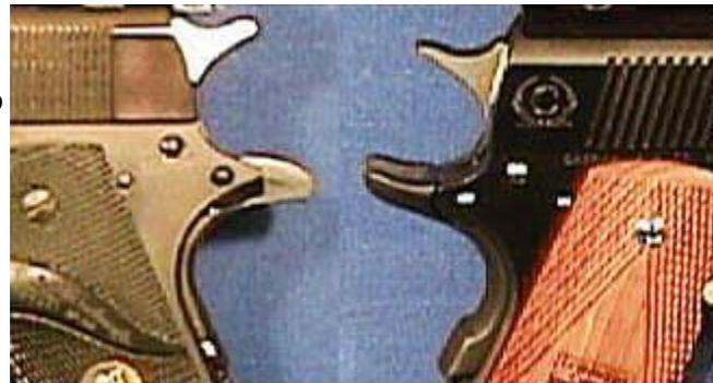
Figure 19: The customers personal tastes dictate the details such as stock or high-rise grip safety.
