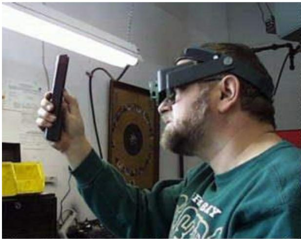
Figure 14: The human eye is the best tool to gauge the fit of the barrel hood in the slide.
