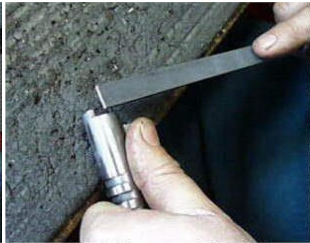
Figure 15: Very judicious removal of metal with an extremely fine Swiss pillar file for fitting barrel hood.
