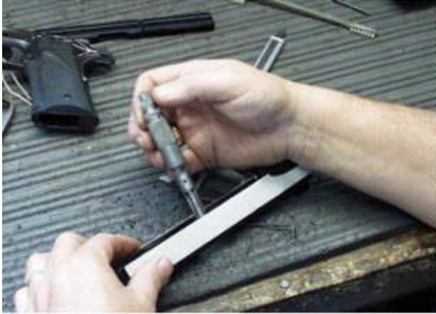
**Figure 10: Using a custom-made micrometer to measure slide rail height.**
