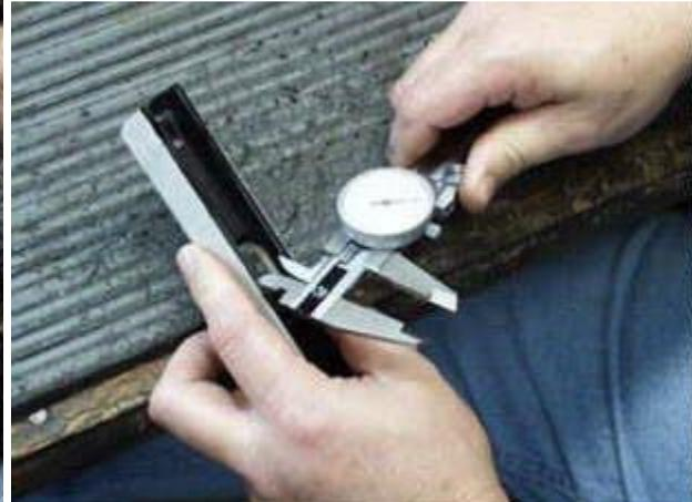
**Figure 9: Slide rail width measurements are also taken at several points**
