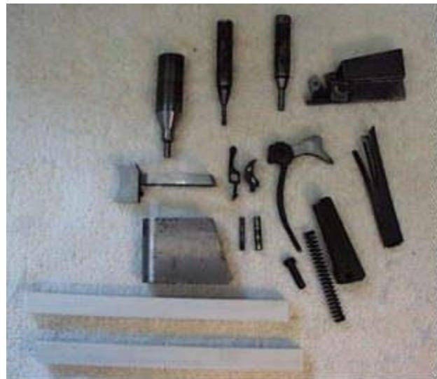
Figure 17: All of the components that affect trigger pull and some of the tools and stones required for fitting and adjustment, not including vises, hammers ...
