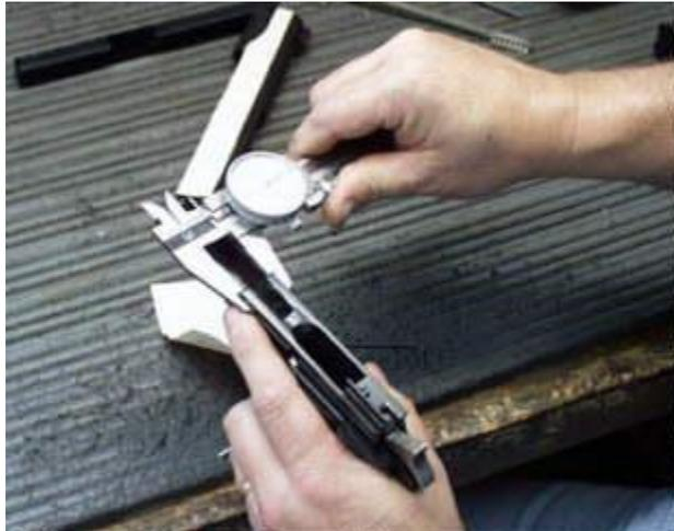
**Figure 8: Frame-groove-width measurements are taken at several points.**
