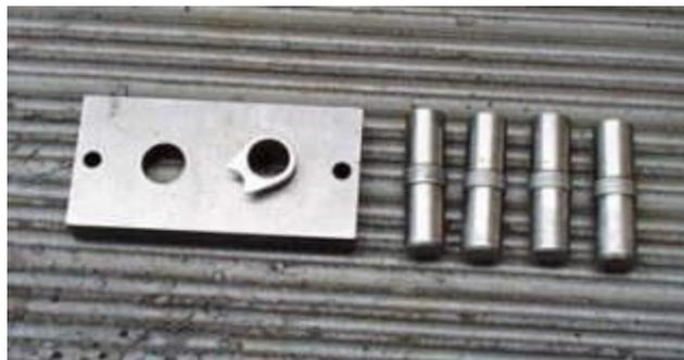
**Figure 13: A National Match bushing in the fixture plate and different expanders to fit the bushing to the slide.**
