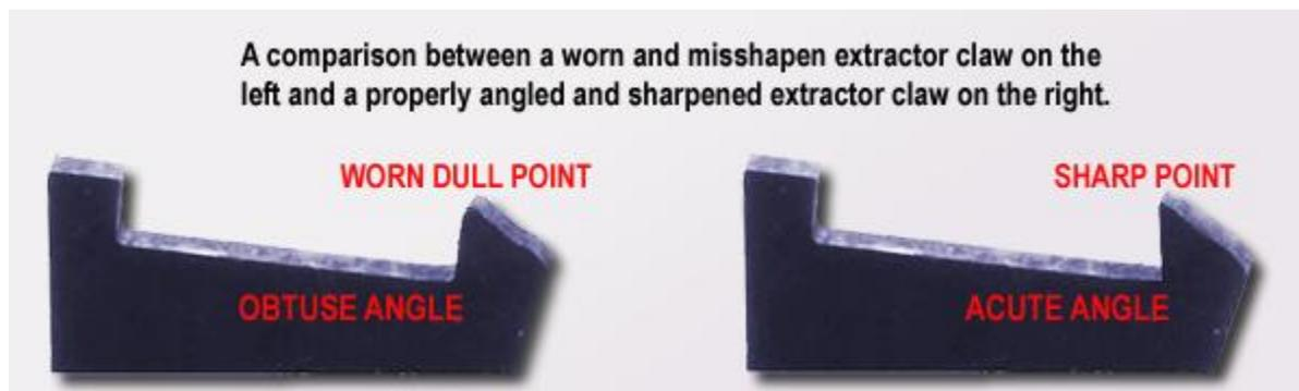
As shown above on the left, this worn and misshapen extractor will clearly not hold the newly spent case in its proper position at ignition. Replacement with a new extractor claw would be the solution - but the new extractor will need to be prepared by checking and adjusting its dimensions against the old extractor and honing the claw a sharp point with a file or other abrasive.
