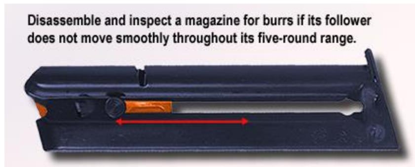
form on the inside of the magazine during the manufacturing process. These burrs can make contact with the internal spring or follower and cause it to stutter. This stuttering will cause a feeding problem.
